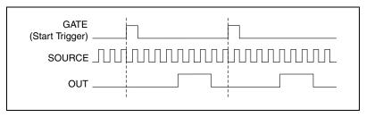
Figure 7-24. Retriggerable Single Pulse Generation
